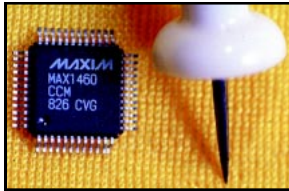
Photo 1—They call it a smart ADC, and the MAX1460 arguably represents Maxim's first entry into the micro market.
