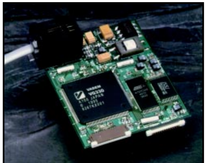
Photo 1 —The Vadem IPump reference design uses their VG330 PC-on-a-chip to enable EPCs to get a piece of the Internet-appliance action.
