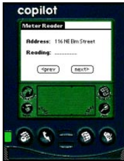
Photo 1—The CoPilot is a virtual PalmPilot on your computer screen that can be used to test applications without downloading to a physical device.
